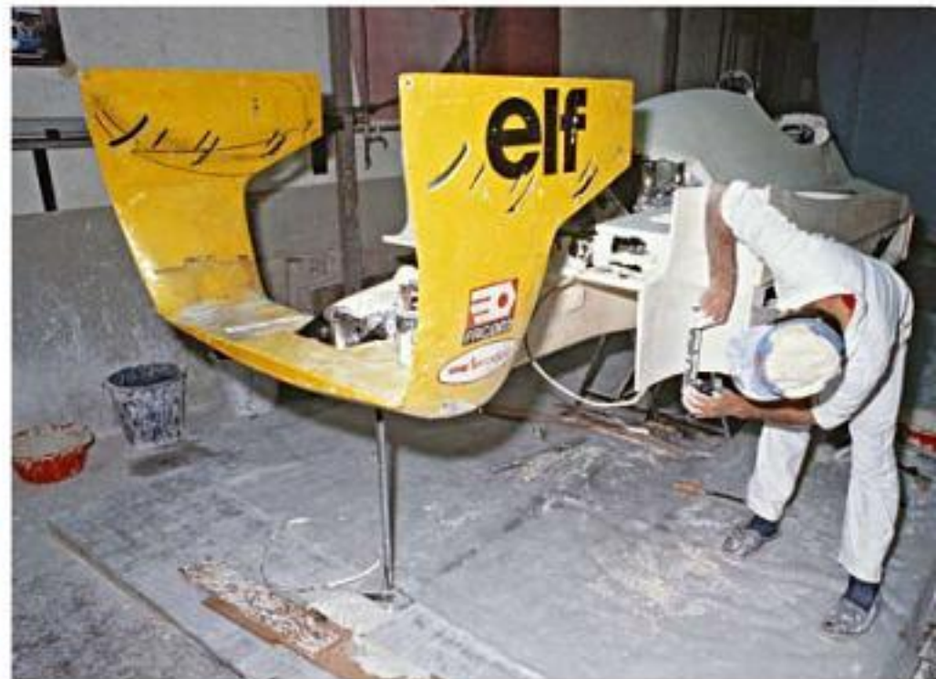
Shaping the moulds.
