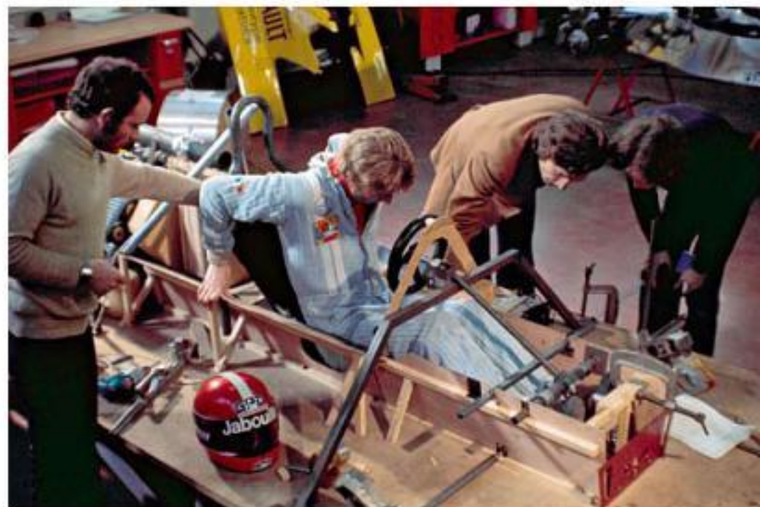
Getting out without becoming stuck or fouling anything is as important as getting in and sitting comfortably. Clearances are measured.
