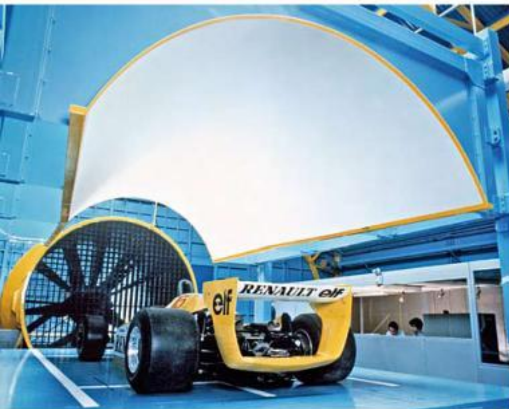
Wind tunnels were quite basic, then! This is the open Eiffel wind tunnel.
