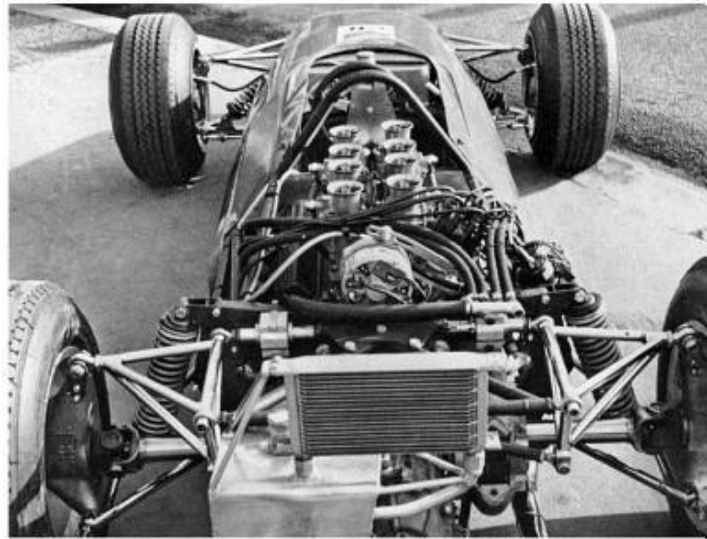
This rear view of the A350 shows details of the suspension, in particular, the two tubular tetrahedrons which serve as upper arms, right and left. (Archives AAA Dieppe)
