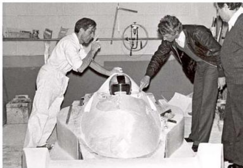
RS01: moulding the master, February 1977, Messieurs Jouvenot, Jabouille, Hubert.
