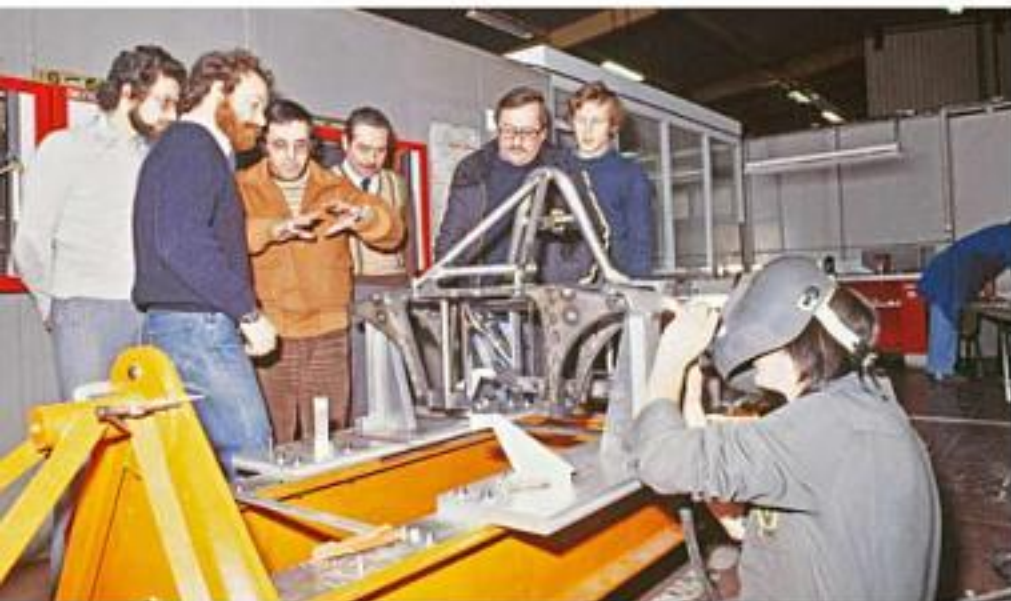
Rear chassis checks. Calculations now play a greater role than the 'suck it and see' approach of previous years.
