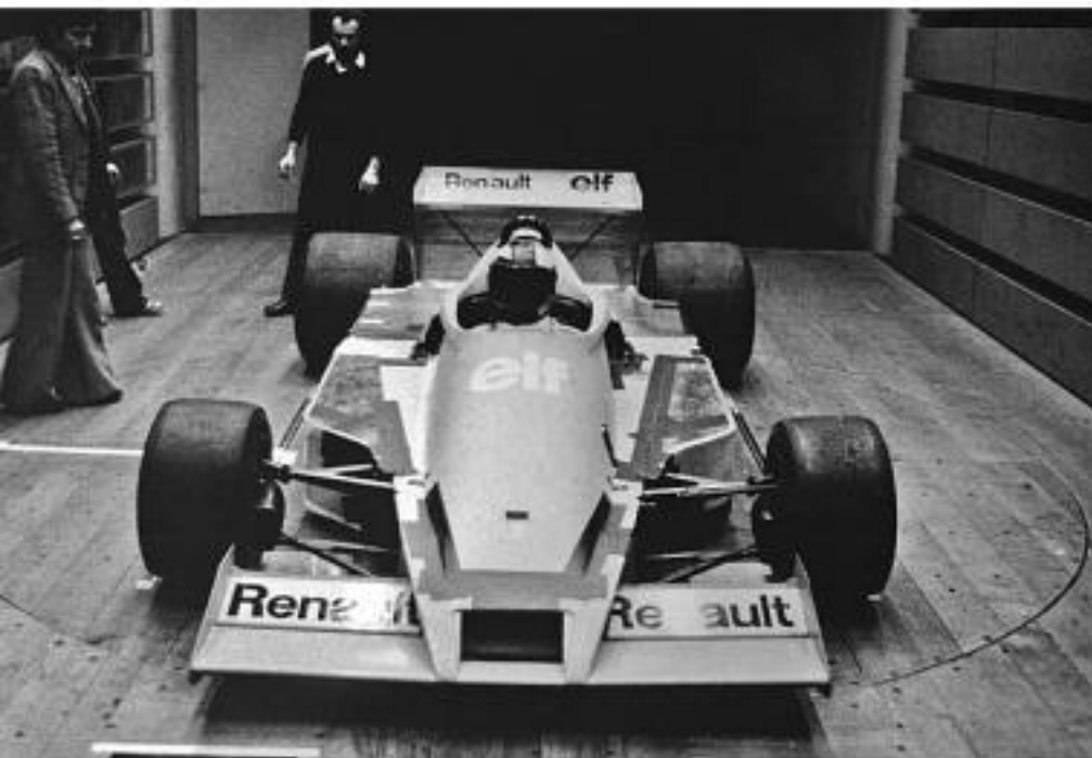
Revisions and trials. Note the taped-on panels over the side-pods. (© Dominique Pascal)
